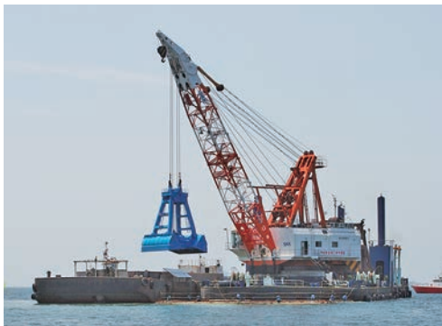
Dredging Vessels with Enclosed-type Grab Bucket
